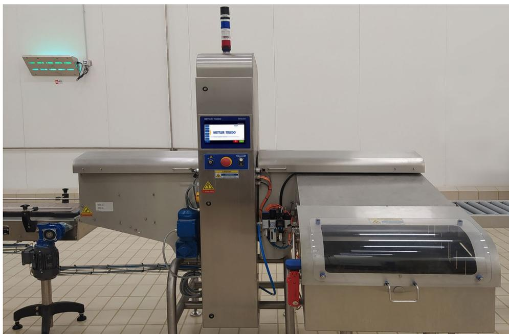
Yogurt products are run through the Safeline X34 X-ray Inspection system to check for any possible contaminant
